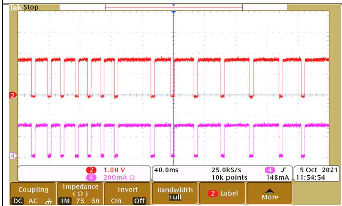
Fig 5.  $V_{IN} = 5V$ ,  $V_{OUT} = 1.8V$ , heavy load OTP
